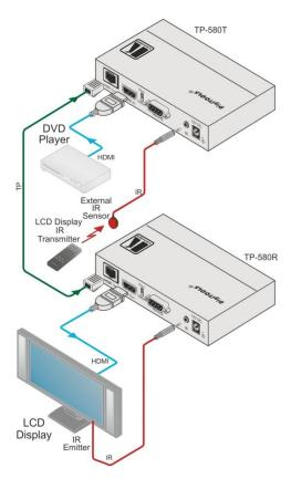
Figure 6: Controlling an LCD Display via the TP-580T
