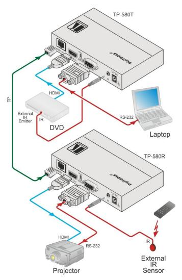
Figure 4: Connecting the TP-580T/TP-580R Transmitter/Receiver Pair
