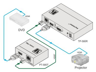
Figure 8: Connecting the PT-580T/TP-580R Transmitter/Receiver Pair
