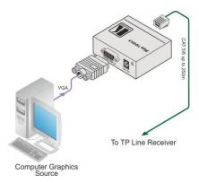
Figure 2: Connecting the PT-110xl UXGA Line Transmitter
